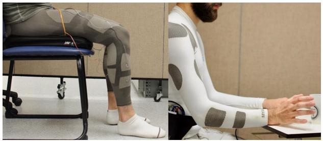
**Figure 1:** Functional electrical stimulation garment prototypes for lower-limbs and upper-limbs motor rehabilitation.
