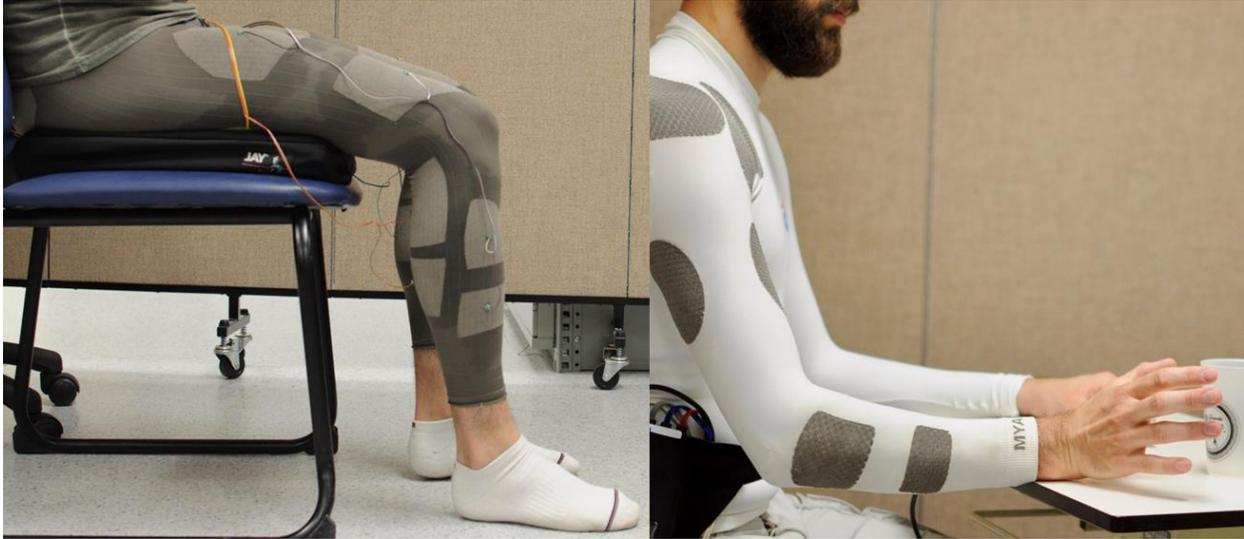
**Figure 1:** Functional electrical stimulation garment prototypes for lower-limbs and upper-limbs motor rehabilitation.
