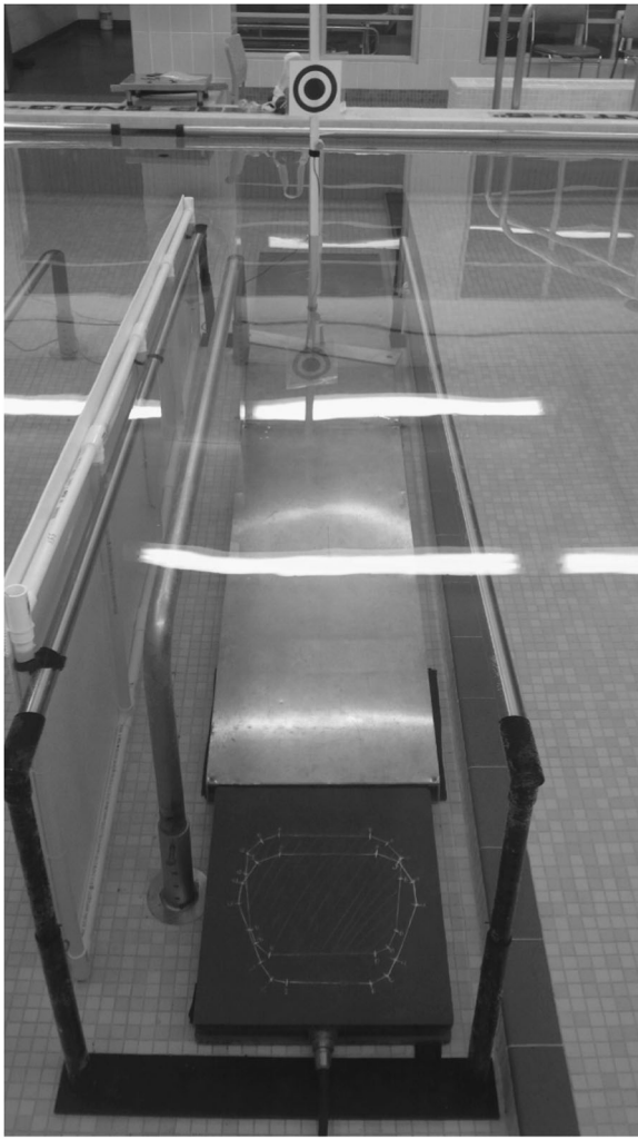
Fig. 1 Experimental set in a therapy pool measuring 9.80 m long, 4.90 m wide and 1.10 m deep (deepest end). The experiment occurred in the deepest end of the pool. Participants stood on a waterproof force plate (0.50 × 0.46 × 0.08 m), within demarked feet contour, in all trials in water and on land. The figure displays the feet contour for two participants. When standing with eyes open, a target was placed at 2-m distance away from participants
